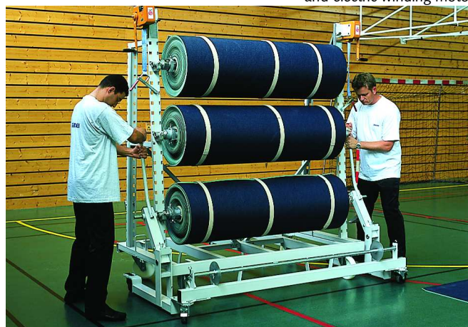
hanging the rolls into the rack with the off- and onrolling device
