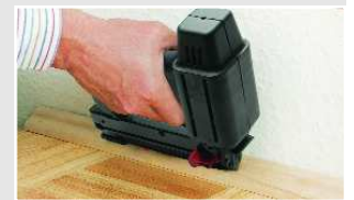
Using the ME 30/08 for almost invisible countersinking of brads when fixing skirting boards
