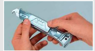
The blade chamber is securely locked and the knife is ready for use
