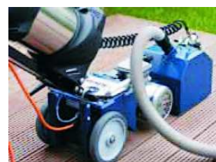
Connection of an external dust extractor
