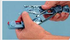
Insertion of the new blade.
