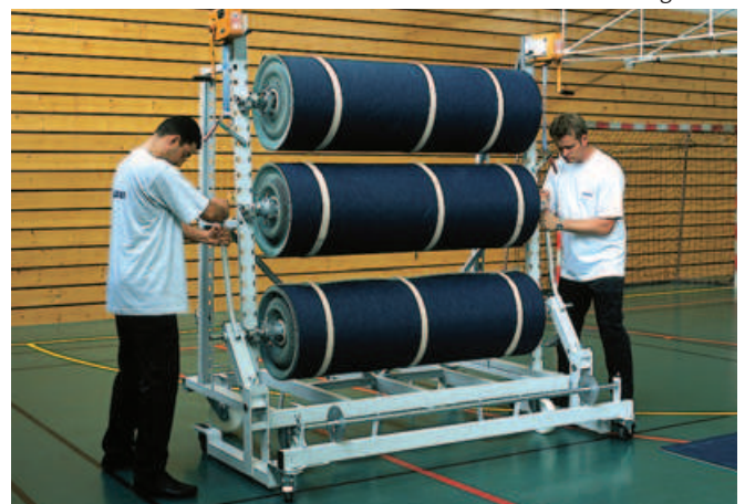
hanging the rolls into the rack with the Transport and Unroll Trolley
