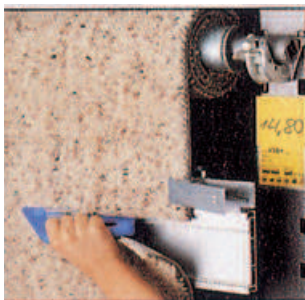
Cutting at roll stand with USF. A fixing clamp and hand cutter are also pictured.
